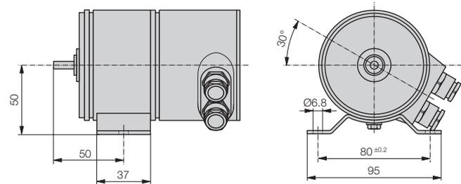
Fig. 13. Fixing with mounting foot.
