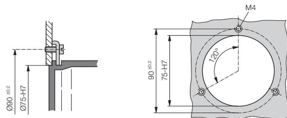
Fig. 12. Left: Fixing with clamps
