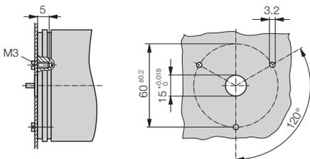
Fig. 8. Left: Fixing with cheesehead screws
