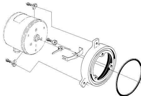
Fig. 14. Accessory kit for pressure gauge mounting (see "Feature 12.")
