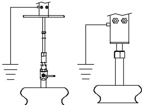
□ **Sensor Installation – Model For Mounting In Not Pressurized Pipe**
