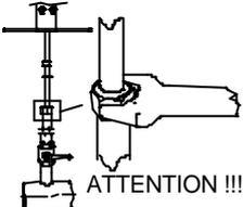
Before opening the ball valve lock the centring bush with the grain in endowment
