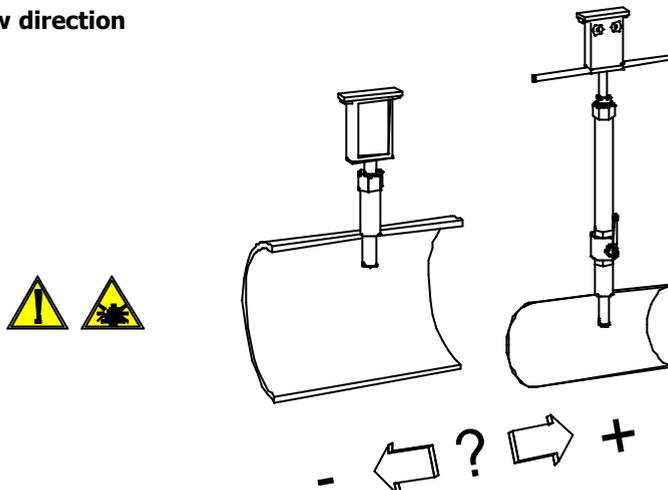
Before install the sensor locate the direction of the liquid in the piping
