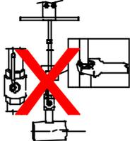
The opening of the ball valve before tighten the fixing nut could cause the expulsion of the sensor from the pipe line
