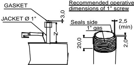
weld the jacket to to the pipe line
