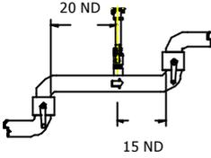
Install the sensor away from curves and hydraulic accessories
